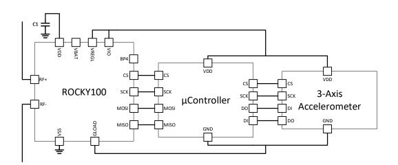
The ROCKY100 IC includes the RF frontend for UHF RFID power harvesting and communication, a power supply module to generate the required voltage levels, and an EPC C1G2/ISO18000-6C digital processor including a SPI bridge. The SPI bridge can be controlled via EPC C1G2 standard memory access commands.
